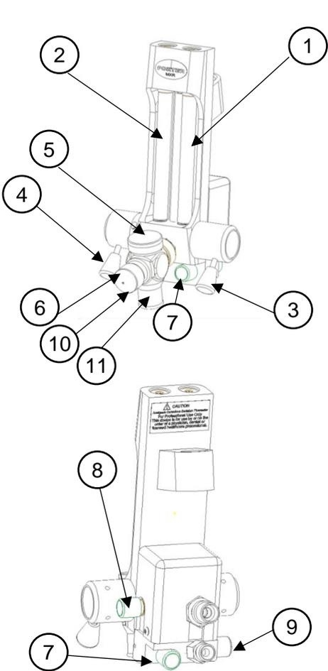
The diagram shows two views of the MXR Flowmeter. The top view is a perspective drawing of the upper section, showing the two vertical flowmeter tubes (1 and 2), the control knobs (3 and 4), and the emergency air intake valve (5). The bottom view is a perspective drawing of the lower section, showing the O<sub>2</sub> flush button (8), the O<sub>2</sub> quick connect (9), and the breathing circuit port (10) and breathing bag port (11). The gas flow on/off switch (7) is shown in both views.
