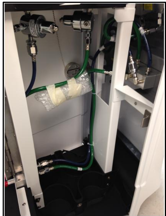
Fig. 19 Hospital Model Hose Assemblies (Inlet Block Assembly lower left)
