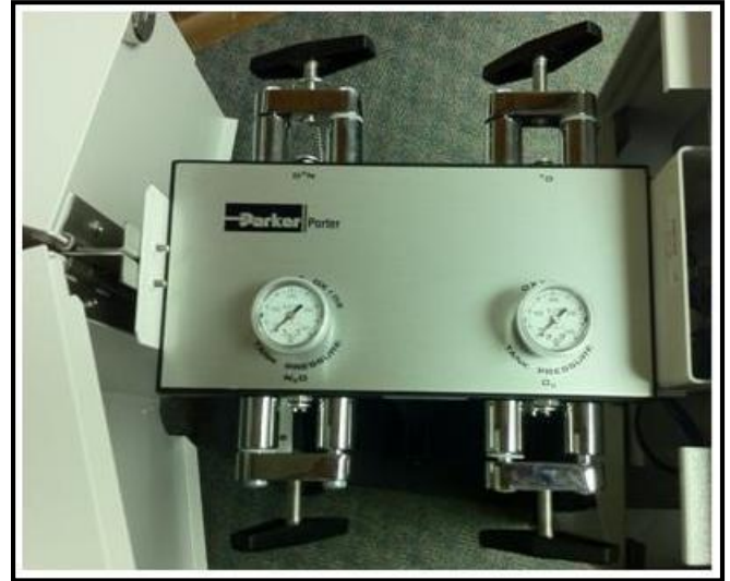
Figure 14 – High Pressure Gauge Locations; E-Block Removal Illustration
